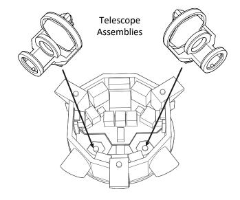
6. Place the Spacecraft Top Assembly onto the assembled Spacecraft Base. Align the pin on the forward Thruster with the forward hole under the top. Then rotate the top so the remaining two holes align with the pins on the other thrusters. If needed, adjust the thruster positions to fine-tune the alignment.
