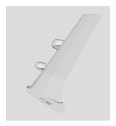
SOFIA is powered by four Pratt & Whitney JT9D-7J turbofan engines, rated at 50,000 pounds of thrust each. Two are on the right wing, and two are on the left.
