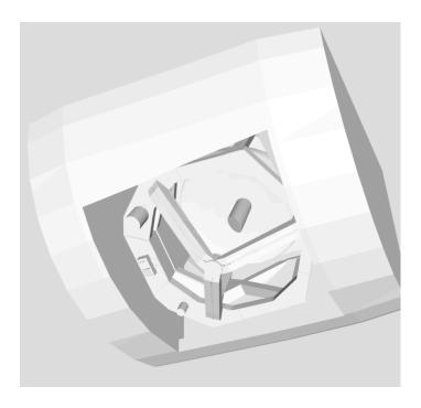
SOFIA's 2.7-meter (106-inch) diameter telescope was built in Germany by MAN Technologie AG and Kayser-Threde GmbH. The telescope collects radiation with wavelengths between 0.3 and 1600 microns and has an altitude range of approximately +20 to +60 degrees above the horizon. The telescope cannot point down.
